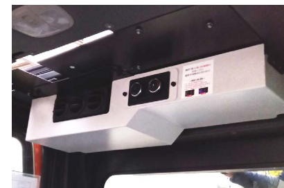
Improvement measures for supplier safety actions (Installation of air conditioners and heaters in electric forklifts)
